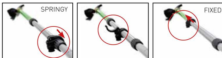
With the moveable locking mechanism the pole can quickly and easily change from springy to fixed pole in just seconds. Note! The locking of the pole can be adjusted by twisting the turning nut so that it is secured on the middle part of the pole. This will guarantee the pole from collapsing and staying in the fixed position.
